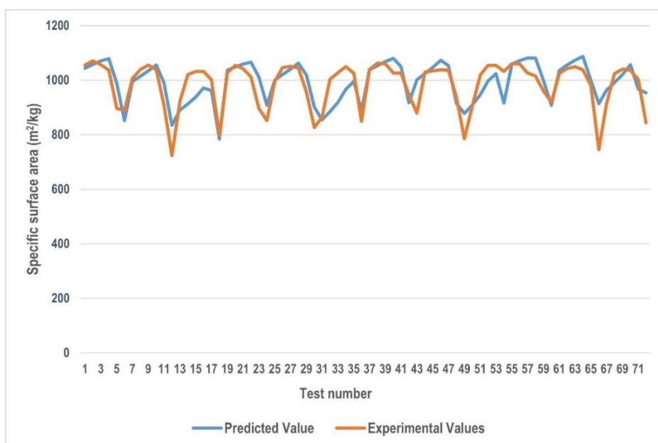
Figure 4 Comparative values of specific surface obtained experimentally and using the ANN model [26]
